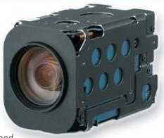
with a variety of convenient features such as spherical privacy zone masking, Electronic-Flip, Picture Freeze, and Auto IR-Cut Filter Removal, all of which have been inherited from Sony's current FCB-EX Camera Series.
