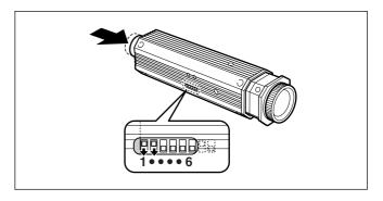
Push the back panel and the CCD head block back into their previous positions, and tighten the Philips screws (7) to a torque of 0.18 N•m.
