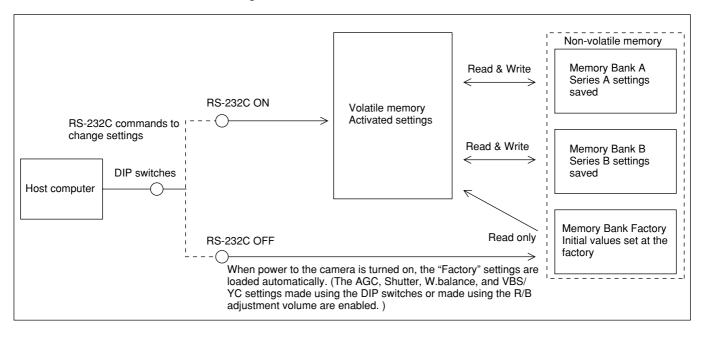
The XC-555/555P is equipped with three Memory Banks (Factory/A/B) to hold camera settings. Factory is "read only," holding the settings made when the camera was shipped from the factory. A and B can be written to, as well as read from, and the user utilizes these locations to hold setting values, calling them up when needed.
