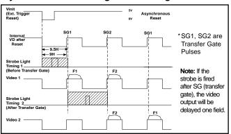
**Strobe Light Timing 1:** Strobe light fires before transfer gate pulse SG1. Both fields of the CCD array are exposed. SG1 transfers out first field F1 (may contain unfinished image from previous field before reset), and SG2 transfers out second field F2.
