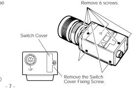
Lens mount should be as shown in the diagram, other-
