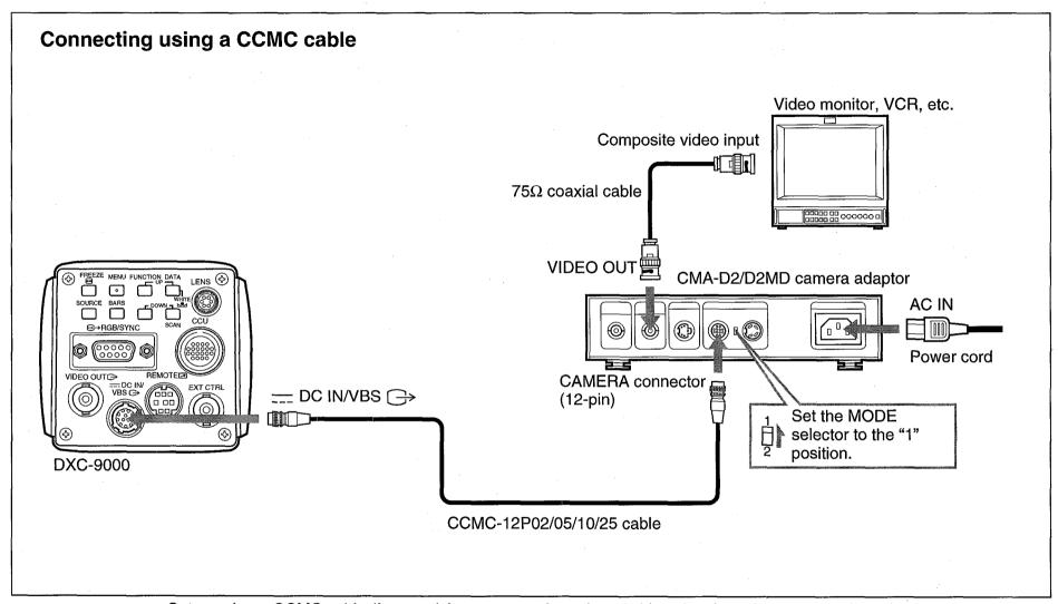
Setup using a CCMC cable (for supplying power to the unit and video signals to the camera adaptor)
