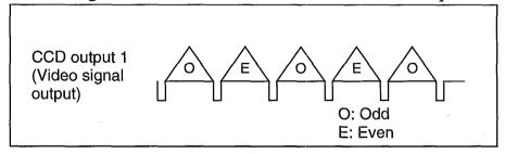
One channel of the CCD outputs is used. The video signal is output from the camera without passing through the memory. Odd-field and even-field video signals are output alterntely.
