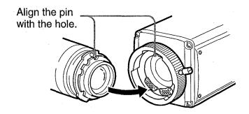
3 Turn the mount lever clockwise as far as it goes to lock the lens in the lens mount.
