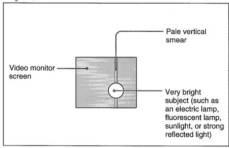
This phenomenon is common to CCD imaging elements using an interline transfer system, and is caused when an electric charge induced by infrared radiation deep within the photosensor is transferred to the resistors.
