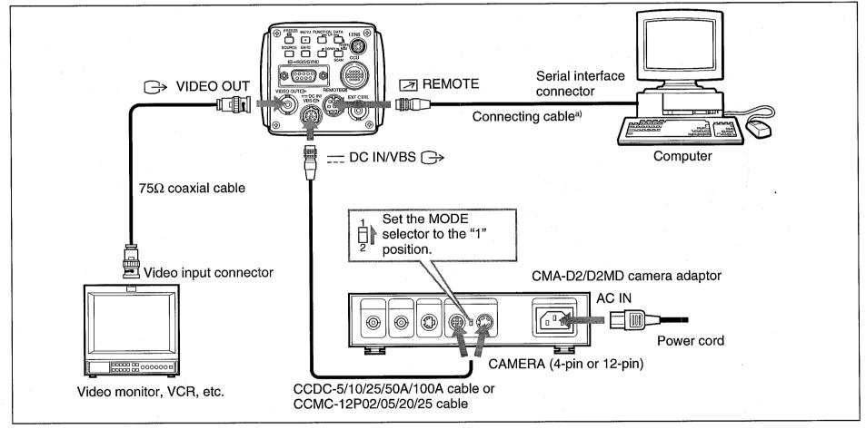
a) Use the shielded connecting cable for connecting to a computer.
