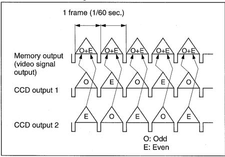
The odd-field signal and even-field signal are sent to memory together and processed as a one-frame video signal in within one field. The video signals for 60 frames are sent in a second. Thus, the unit can output twice the video signal that can be output from a conventional unit.
