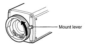
Align the positioning pin on the lens with the matching hole in the lens amount and attach the lens.
