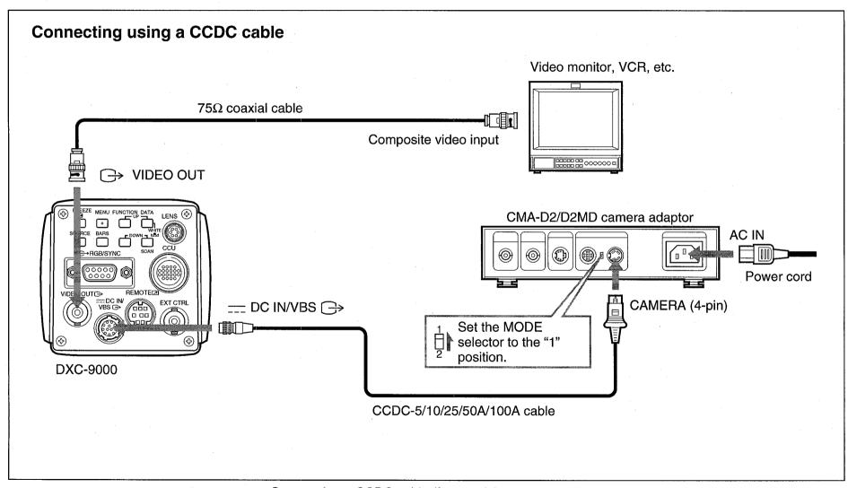
Setup using a CCDC cable (for supplying power only)
