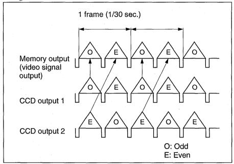
The odd-field signal and the even-field signal are sent to the memory together and they are interlaced in memory and output as the video signal for one frame.
