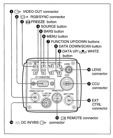
Outputs RGB signals and their respective sync signals. Use a CCXC-9DB/CCXC-9DD/CCMC-9DS cable for the connections.
